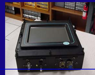
BRIDGE CONTROL PANEL
